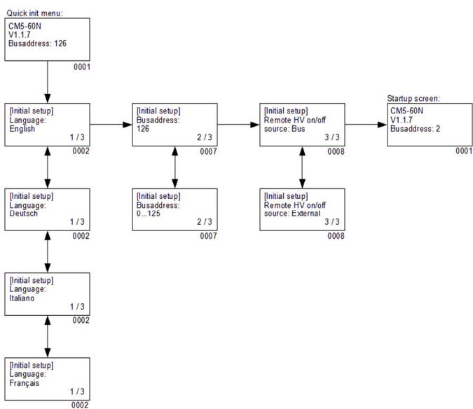
The ‘Initial setup’ or quick configuration menu is used to quickly configure the generator. The generator can be used immediately after configuration.
