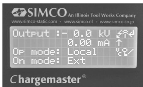
The main screen of the generator shows the currently measured voltage and current and also the operational mode. Texts are shown on the left-hand side of the display and symbols on the right-hand side. The symbols that refer to an operational mode appear on the same line as the text.
