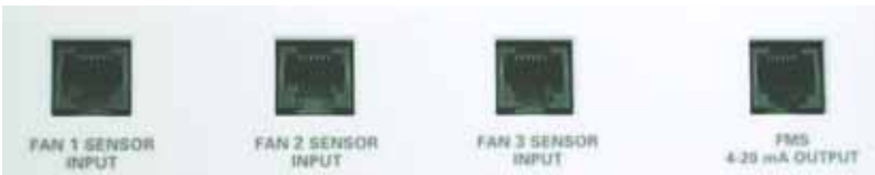
Figure 14. Close Up of Sensor Inputs for Fans 1-3 on a 3-fan Unit
