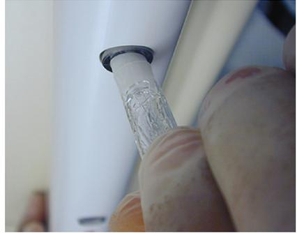
Figure 10. Cleaning Points with the Emitter Point Cleaner
