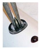
Figure 15. Removal of Silicon Emitter Point
