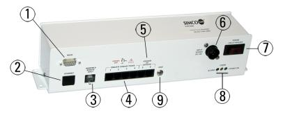
Figure 2. Interface Module Model 5200-IM6T
