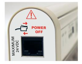
Figure 6. CAT-5 Cable Connection
