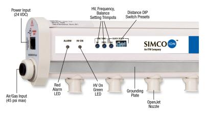
Figure 1. Model 5635 AeroBar MP with Open Jet Nozzles
