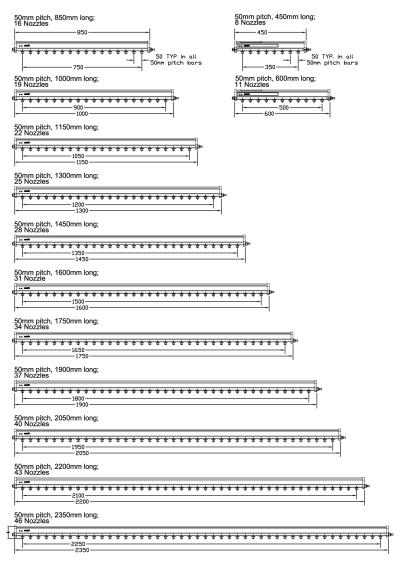
Figure 10. Model 5635 Lengths with 50 mm and 75 mm Emitter Pitch Spacing
