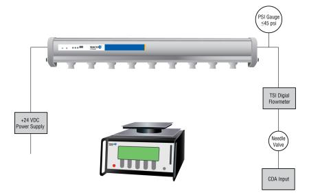
Figure 9. Recommended Setup for Calibration
