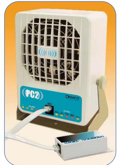
LED status indicators on the front of the PC2 provide monitoring of the following critical functions: Power, Ion Output, Ion Balance, System Fault, Stalled Fan, and when Emitter Service is required before the emitter condition affects ion output.
