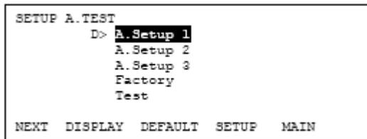
A symbol "D>" indicates which one is selected as the default test. To change the default, scroll to highlight one of the options using the
