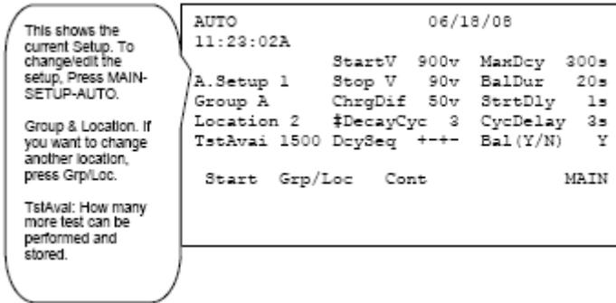
This shows the current Setup. To change/edit the setup, Press MAIN-SETUP-AUTO.
