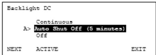
The backlight of the display can be set to continuous lighting or shut off in 5 minutes when it is using battery.
