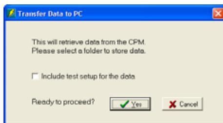
checking “Include test setup for the Data”, will also download the test setup information from the CPM. Click
