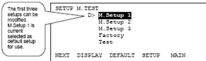
This screen displays a list of five user selectable manual test options. Three of them; M.Setup 1, M.Setup 2 and M. Setup 3 may
