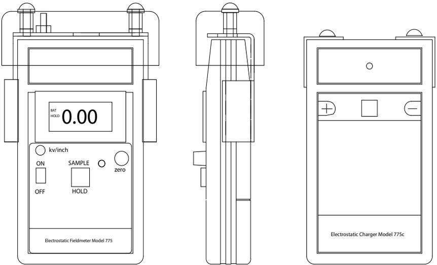
Model 775 Fieldmeter with Model 775P Plate Assembly
